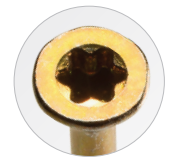
Deep T-25, 6-lobe recess provides improved control and greater bit life
