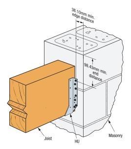
**HU Fix on Masonry Installation**
