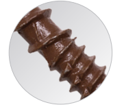
Inverted Upper Threads clear excess material to ensure the screw is seated properly and consistently
