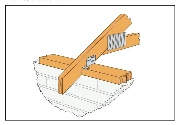
In all circumstances, the GS should be fixed by even hammering to a 100mm horizontal cut made in the rafter so as to allow proper bearing over the wall plate. The location and cutting of the notch in the rafter should be approached in the normal manner i.e. as if no GS was being installed so as to provide a level bearing surface for attaching the upper bearing plate.
