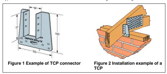
The Miscellaneous Brackets and fasteners are made from zinc-coated steel or stainless steel and are available in various sizes. Annex 2 contains the Miscellaneous Brackets' full range description.
