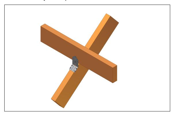
Position VTCR onto the common truss ensuring the timber is of adequate width to accommodate the specified fasteners and ensuring the connector is positioned in the centre of the truss width.
