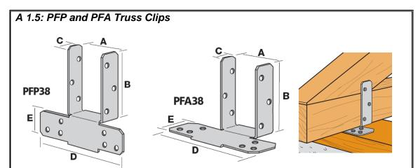
Table 6: Specifications of PFP and PFA Truss Clips.
