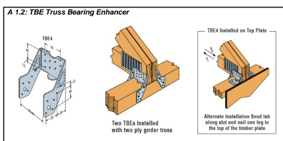
Table 3: Specifications of TBE Truss Bearing Enhancer
