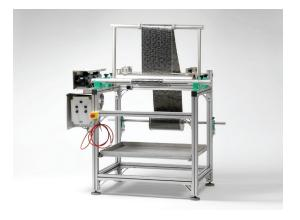
In case of larger quantities use S&P wet-lay-up machine for pre-impregnation.
