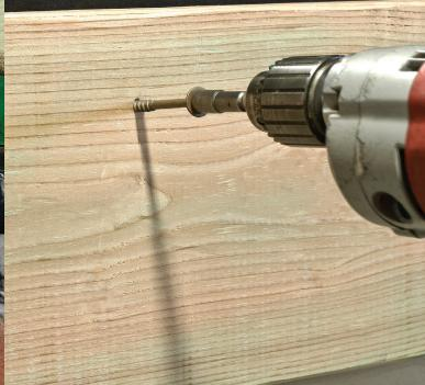
Superior to nails in holding power and pullout resistance
