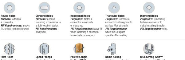
Tooling holes for manufacturing purposes. No fasteners required.
