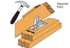
**STEP 3:** Install "B" flange nails in the obround nail holes, locking the pitch.
