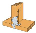
STEP 2: Use speed prong to temporarily hold A35 in place. Install nails as shown.
