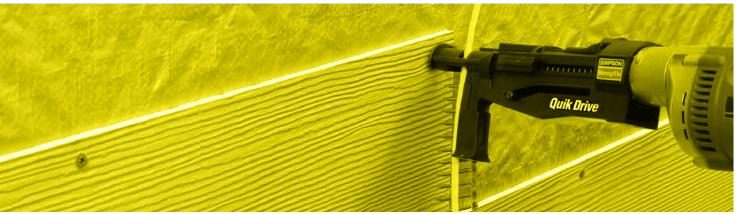
The WSCBGHLA114SA is designed for cement board-to-steel (0.55–0.75 mm) applications with its sharp point and high-low thread design. Whereas the WSCBGA158SA with its Type 17 point and coarse thread is designed for cement board-to-timber applications.
