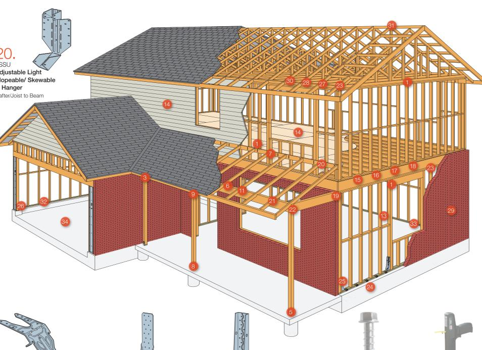
31. Ridge Rafter Connector Rafter to Ridge Beam
