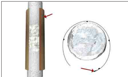
Install a bead of FX-763CTG into the locking groove of the jacket and place FX-70® jacket around the pile to be repaired.
