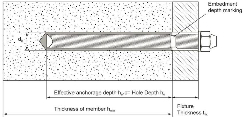
**Anchor application in hollow/perforated masonry with nylon sleeve (brick n°2 according to Annex B9)**
