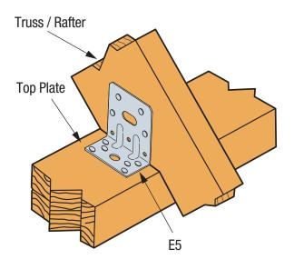
SIMPSON Strong-Tie® E5 Rafter/Truss-to-Top Plate Installation
