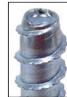
Serrated teeth on the tip of the Titen HD® screw anchor facilitate cutting and reduce installation torque.
